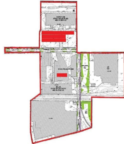
Drainage area map showing the 31.85-acre area that drains into the green shaded Cortex Commons stormwater treatment practices.
